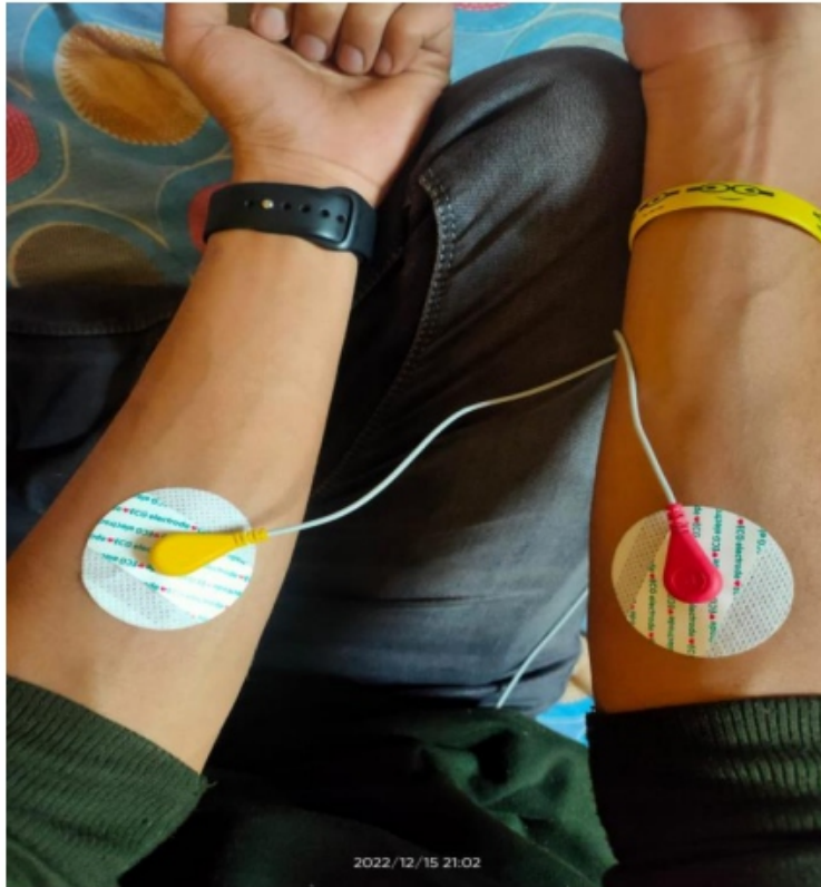
Figure 10 ECG Electrode Placement on Hand
